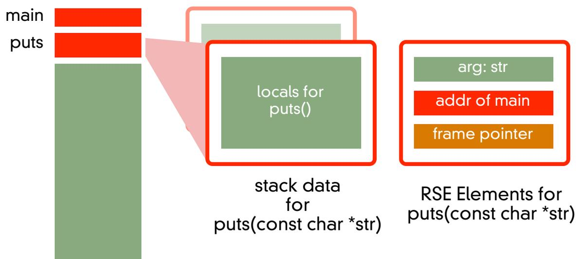
Under SourceT, stack control information is passed in the Itanium RSE. The RSE stores the function arguments, and any control information, in a set of registers.<sup>7</sup> Function local variables are still stored in a traditional, memory based stack. The stack itself is non-executable.
