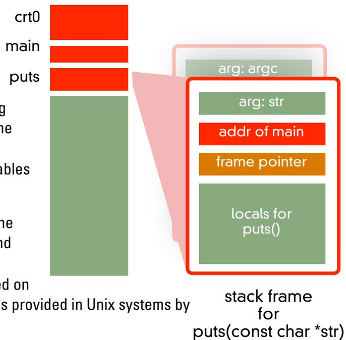
A call by a function to another function causes an additional frame to be generated and pushed on the stack. When a function has completed execution, register and control state for the previous function is restored, and the application continues execution at the address specified on the stack.
