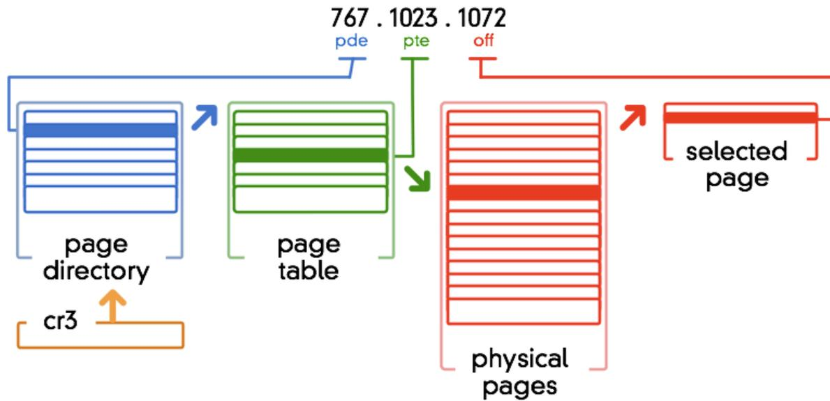
X86 addresses encode a page directory index and a page table index, allowing for 32 bit address mapping in a sparse address space. Operating system processes use the CR3 register to store the location of the page directory, the root of address lookups for each process.
