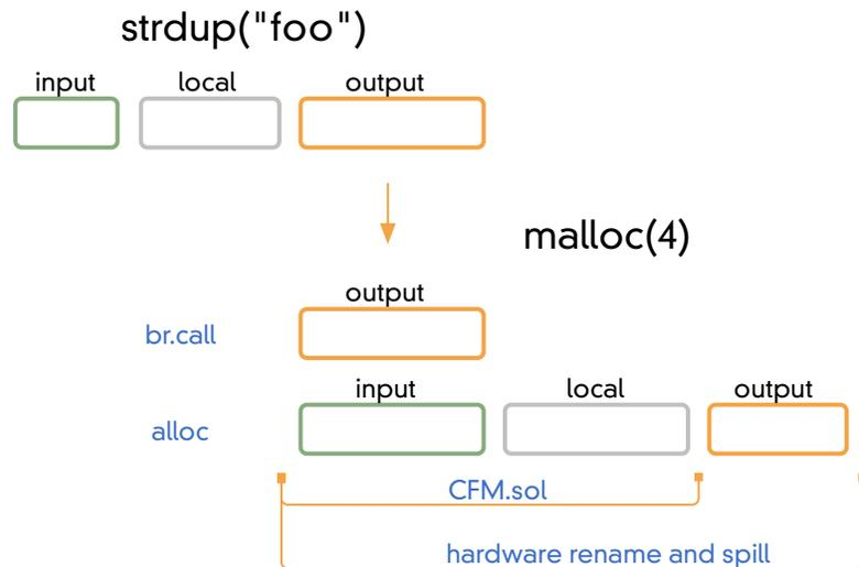
The RSE provides explicit hardware spill and fill. When the dynamic register file is exhausted, the RSE spills GPRs to a region of memory. This memory region can be at a higher privilege level than the function itself.
